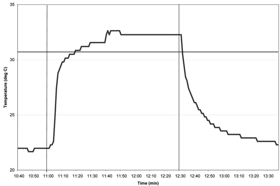
Figure 4. Example of exported data from the StowAway TidbiT with determined cut-off temperature (30.6°C) represented by the horizontal line.
